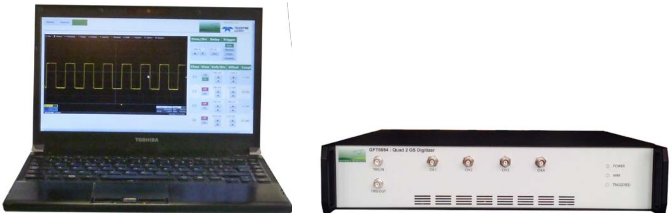
Figure 1: GFT6084 and laptop with embedded web page
