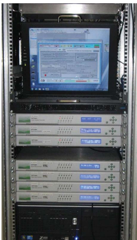
Figure 6: View of LULI timing system. In this installation the users have measured the long-term jitter in a temperature stabilized environment. The results are shown in Figure 7.
